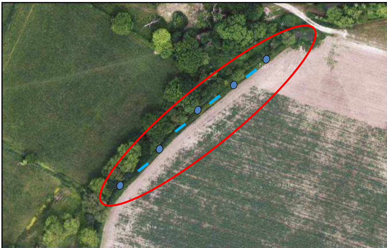
Option B – re-meandering the watercourse to create more natural and dynamic stream with pools, riffles, cliffs and bars
