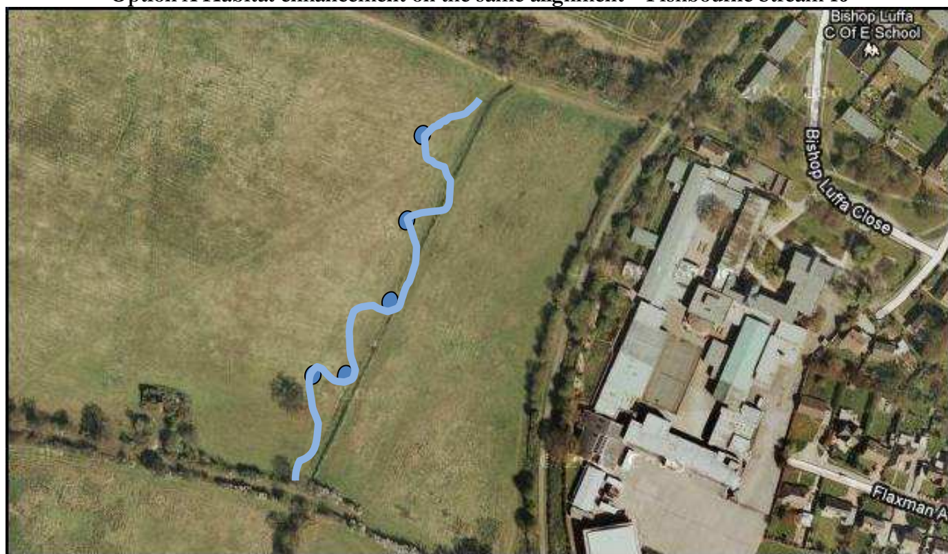
Option B - Habitat enhancement changing the alignment – Fishbourne Stream 16
